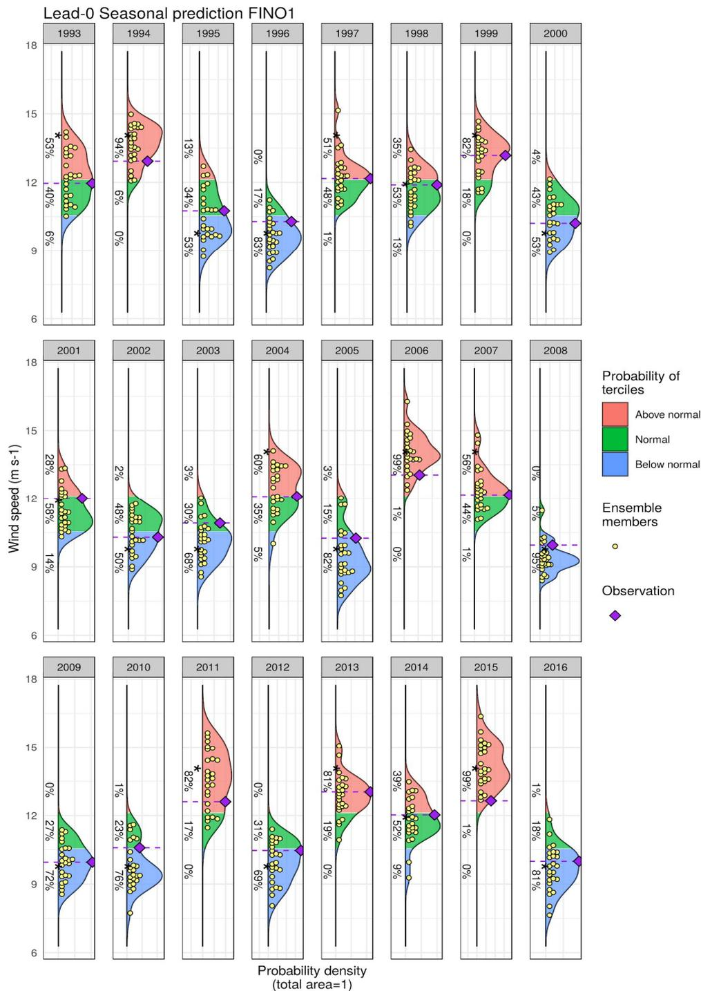
**Figure 1.-** Lead-zero winter seasonal predictions at FINO1 met mast (54.0°N, 6.6° E) for the 1993-2016 period.. The yellow dots represent the values for the 25-member ensemble of the ECMWF SEAS5 prediction, whereas the purple square shows the observed seasonal mean wind speed value at FINO1. The Probability Density Functions have been built by dressing the ensemble members with the Kernel Density Estimate method.
