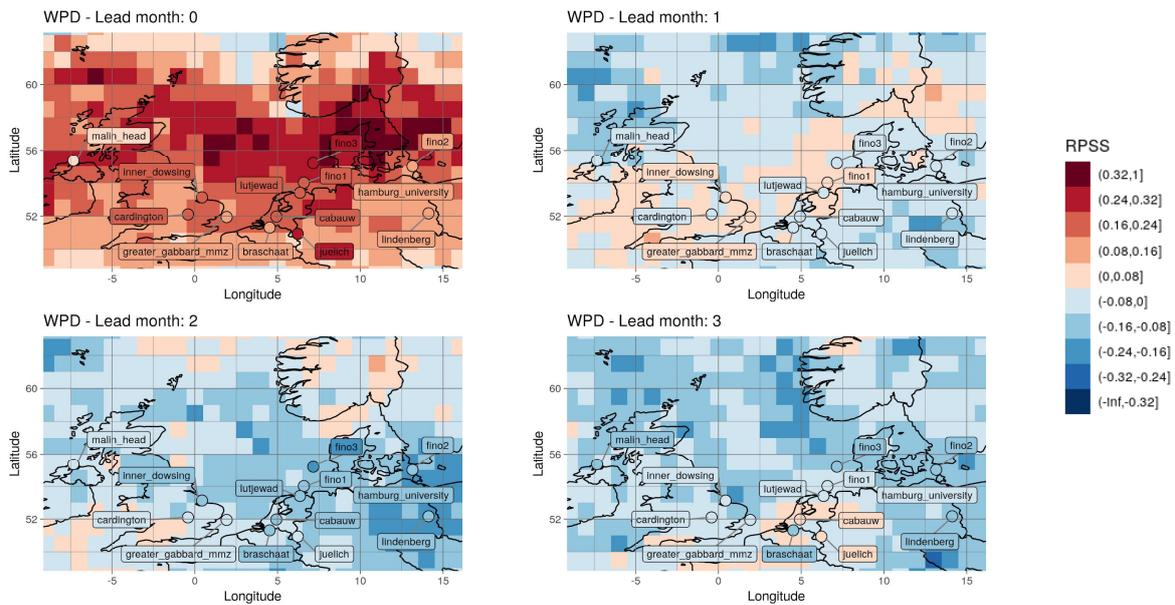
**Figure 5.** RPSS of the WPD SEAS5 predictions in the North Sea region for DJF. Predictions were initialised in December (lead month 0), November (lead month 1), October (lead month 2) and September (lead month 3). Points indicate the RPSS of the predictions at the 17 tall tower locations.
