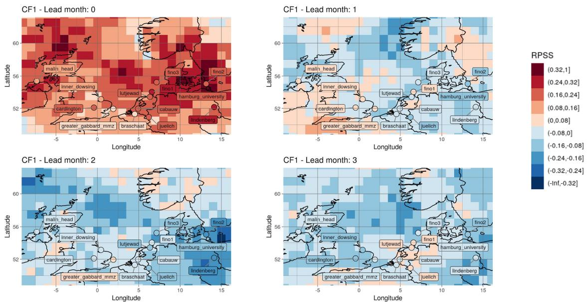
**Figure 4.** RPSS of the CF1 SEAS5 predictions in the North Sea region for DJF. Predictions were initialised in December (lead month 0), November (lead month 1), October (lead month 2) and September (lead month 3). Points indicate the RPSS of the predictions at the 17 tall tower locations.
