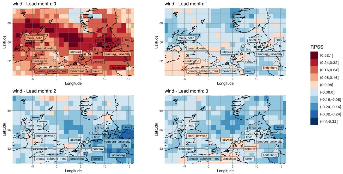
**Figure 3.** RPSS of the hub-height wind speed SEAS5 predictions in the North Sea region for DJF. Predictions were initialised in December (lead month 0), November (lead month 1), October (lead month 2) and September (lead month 3). Points indicate the RPSS of the predictions at the 17 tall tower locations.
