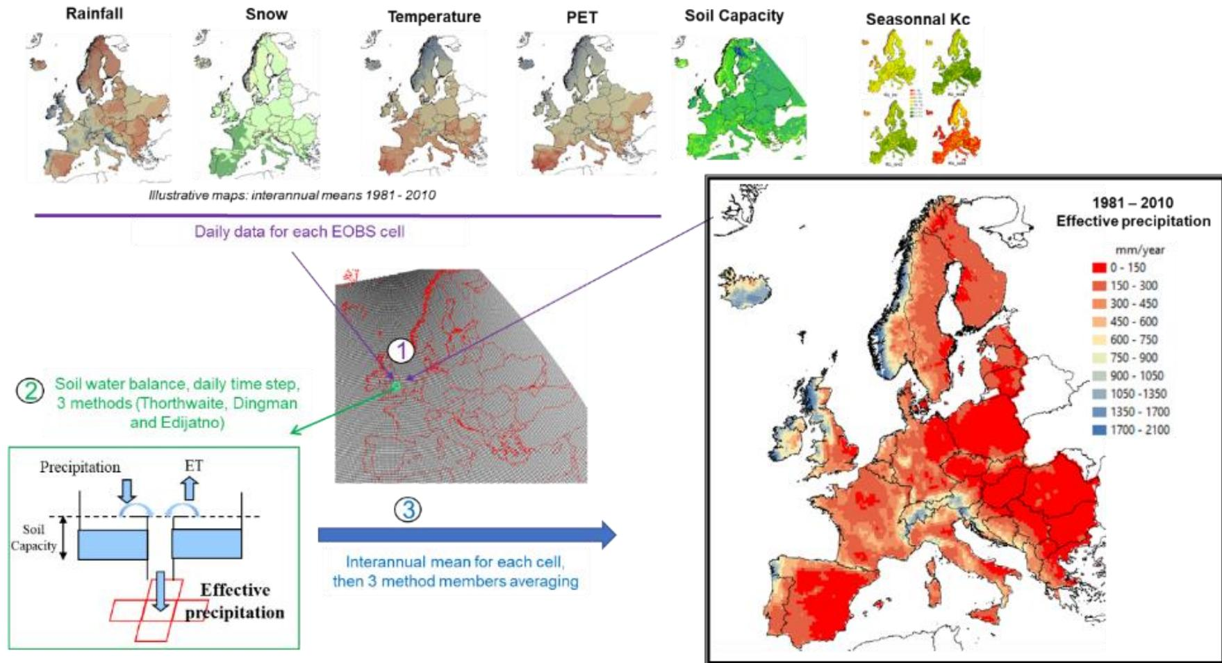
Figure 4: Sketch of the methodology applied to compute effective precipitation at the European scale.
