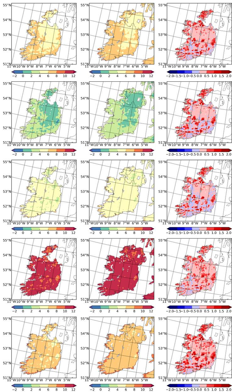
Figure 19: Mean daily temperature minima for the period 1981-2017 inclusive. Unit [°C]
